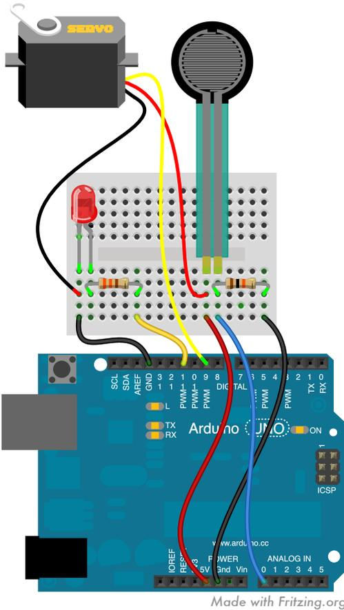
However, the **Servo library** for Arduino takes care of all this. Note the **#import** statement, the **Servo** object declaration, and how the sample code then sends data to the servo using angular values. You can easily declare, create, and control two or more Servo objects this way – essential for your robot!
