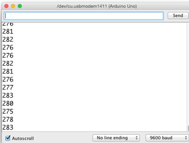
The code uses **Serial.begin(9600)** to open a serial connection back to your computer in `setup()`, and **Serial.println(...)** to output ("print") numbers to that serial connection, which end up in the Serial Monitor window on your screen. It's also possible to send data back to the Arduino that way, using **Serial.read(...)**.
