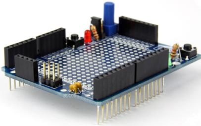
The MAKE Pack contains a kit for a [MakerShield](#) prototyping shield (see photo). **Solder** it together (URL for instructions on the pack), stick the mini breadboard onto it, and you have a very useful board with some built-in LEDs, buttons, even a potentiometer for quick experiments. It's not a perfect fit for the Arduino, but it works well enough. **SparkFun** has a similar [ProtoShield](#).
