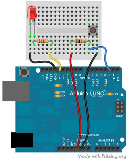
Above the `setup()` function, add `int pushbutton = 2;` At the start of your `loop()` function, add the line `if (digitalRead(pushbutton)==LOW) {...}`. Replace the ellipsis between the curly braces with the rest of the code in `loop()`. Note the double equal sign. Now, the LED will only blink while you press the button and pin 2 is low.
