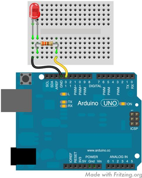
**Disconnect USB.** In the **mini solderless breadboard**, each vertical **column** of 5 holes is **connected** inside the board. Stick the LED, 330  $\Omega$  resistor and jumper wires in as shown. Current will now flow from Arduino **pin 13** through the **resistor** and the **LED** to **GND** when pin 13 is HIGH.
