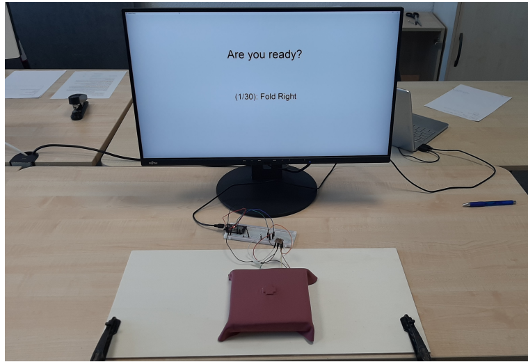
Figure 6.1: The study setup: The Grablet prototype is fixed onto the table before a screen, showing the next gesture the participant is asked to perform.
