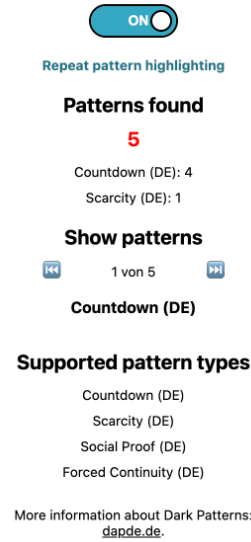
Figure 2.4: Popup of the Dapde Pattern Highlighter 8 browser extension, including the amount of detected deceptive patterns per language (DE). The popup also showcases a list of supported patterns and the ability to toggle the detection.
