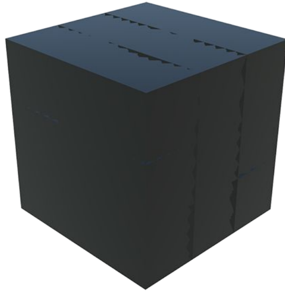
Figure 3.8: Example of emerging artifacts from Z-fighting, created by overlapping nodes
