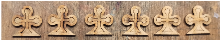
Figure 4.2: Different amounts of removed material depending on lasercutter settings. From left to right, power was successively decreased, while speed was increased.
