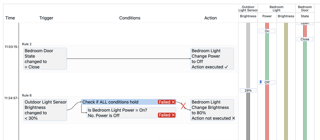
Figure 3.5: Dashboard's Filtered View displays only the relevant rules and devices involved in the success or failure of a particular action.
