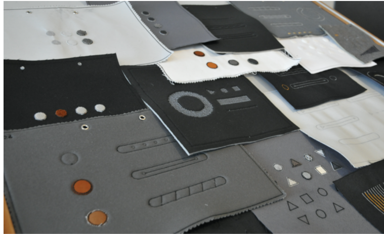
Figure 2.6: Textile Prototypes: Mlakar and Haller used an embroidery machine to create a variety of different non-functional textile prototypes.
