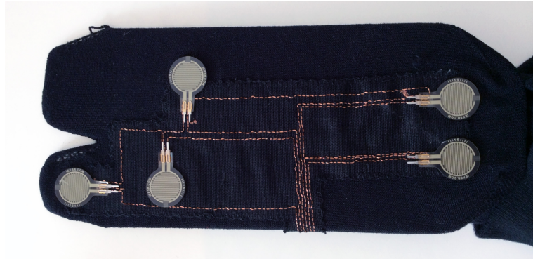
Figure 2.1: Second proof of concept by Goveia da Rocha et al.: Conductive traces were embroidered onto cotton fabric to securely position and solder the FSR sensors. The cotton fabric was then integrated into an off-the-shelf hallux sock.
