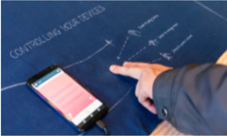
Figure 2.11: Example larger textile interface: Interactive environment on a table designed with Project Jacquard's textile interface by Poupyrev et al.
