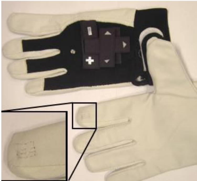
Figure 2.5: Wearable textile interface example: Textile interface integrated into gloves by Holleis et al. Configurable buttons are positioned on the left palm, while the right index finger is used to initiate commands.
