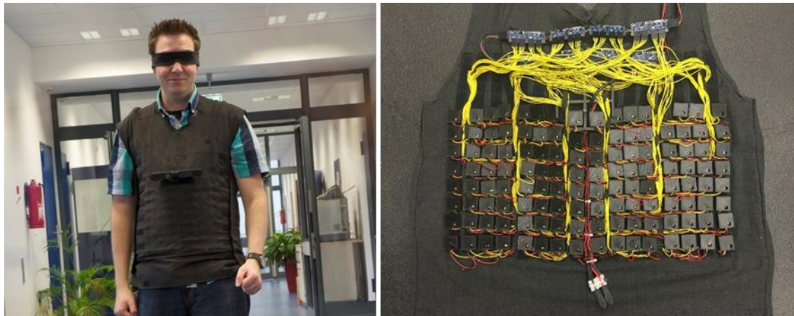
Figure 3. Left image shows a VibroVision vest user, the chest mounted camera provides 3D information that is conveyed via spatialised vibrations arranged in a 16 \times 8 matrix (right image).
