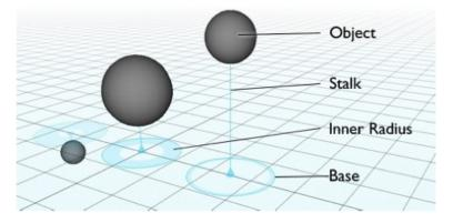
**Figure 6.1:** Composition of position pegs. The pegs provide feedback about object position in relation to the grid. (Image from Glueck et al. [2009])
