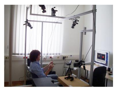
**Figure 4.2:** *Camera constellation as used during the study. The hands were consistently tracked regardless of the orientation.*
