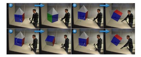
**Figure 2.7:** The four mappings between the hand movement and the rotation of the object. The right hand controls two axes (1, 2) while the left hand controls the third (3). The upward movement of the left hand results in the same rotation as the same motion with the right hand (4).
