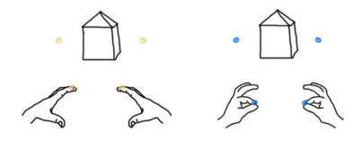
**Figure 4.1:** *Left: Object is released. Right: Object is grabbed. Markers change colour to signify the grabbed state.*
