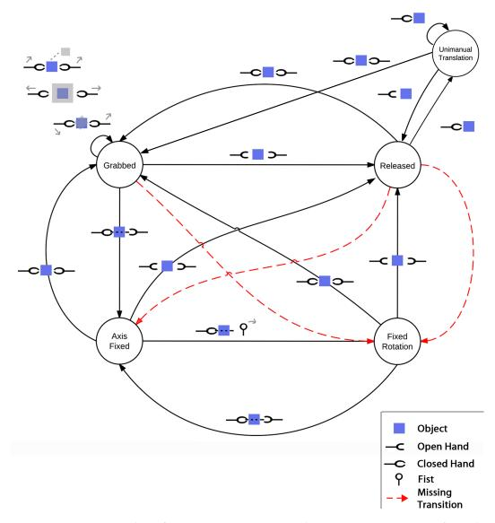
**Figure 3.3:** State machine for gesture transition. Red transitions are missing from the interaction design and represent limitations of BASH.
