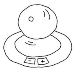
**Figure 2.2:** *The trackball. The user can rest his arm on the table, which stabilises his movements.*
