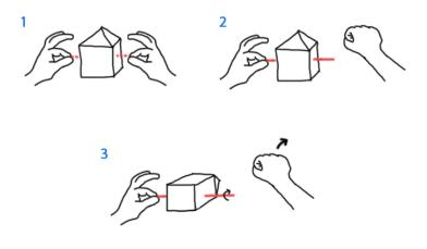
**Figure 3.2:** Gesture for fixed rotation. Left: Object is grabbed in free rotation mode. Centre: One hand forms a fist, which triggers the fixation of the axis. **Right:** Fist performs cranking motion to rotate the object around the fixed axis.
