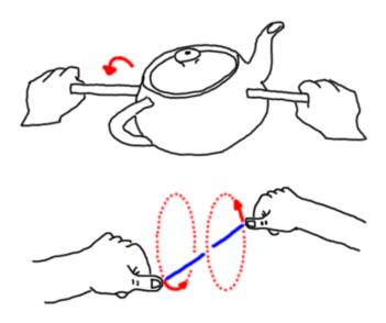
**Figure 2.5:** The "pedaling" motion: incremental x axis rotation using continuous rotation around the y and z axes. (Adapted from Song et al. [2012])
