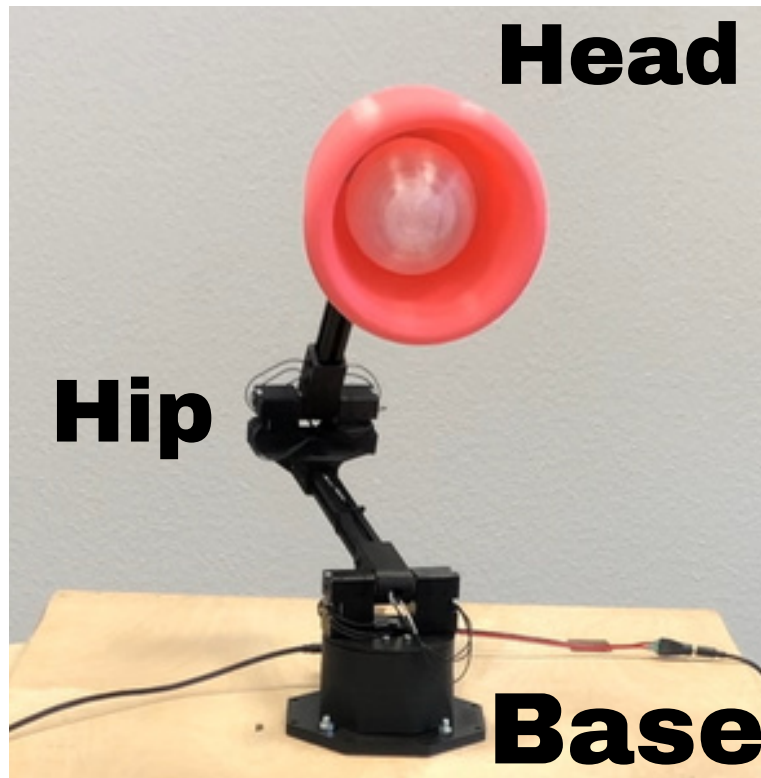
Figure 3.2: The Dancing Desk Lamp - Appearance and naming conventions
