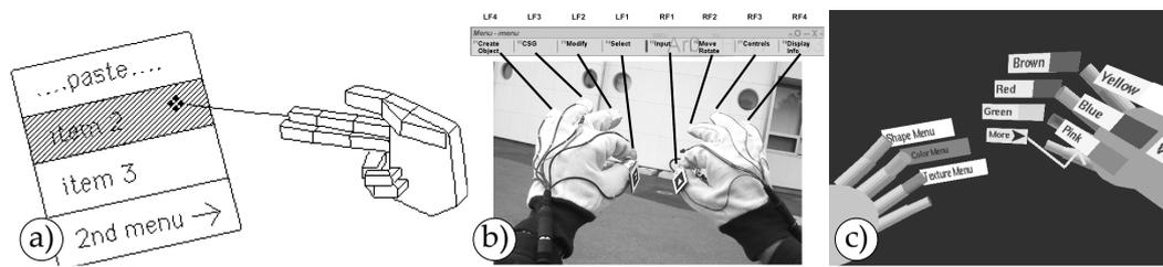
**Figure 2.7:** Gesture-based AR/VR menu techniques by Piekarski and Thomas [2002a] (a), Jacoby and Ellis [1992] (b) and Bowman and Wingrave [2001] (c). The menu presented by Piekarski and Thomas uses gestures to open the menu and create a ray. The menu system of *Tinmith-Hands* (b) and the TULIP menu (c) select a menu item by touching the corresponding finger with the thumb. Images are adopted from the corresponding publications.
