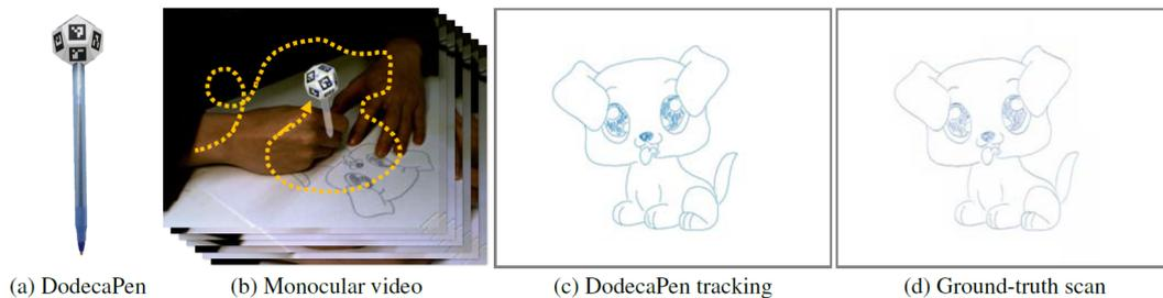
**Figure 2.10:** The *DodecaPen* (a) is a real-time trackable pen (b) with high accuracy (c & d). Image taken from [Wu et al., 2017].
