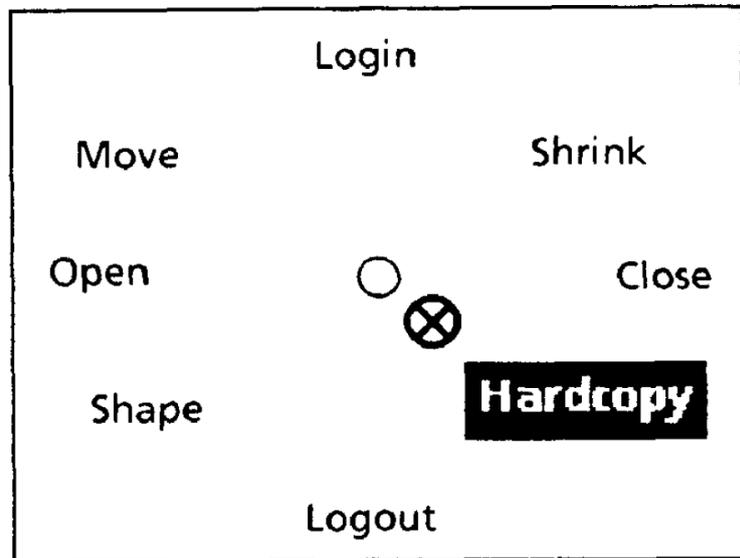
**Figure 2.3:** The pie menu arranges all menu items equally distributed around the user's cursor. Image taken from Callahan et al. [1988].
