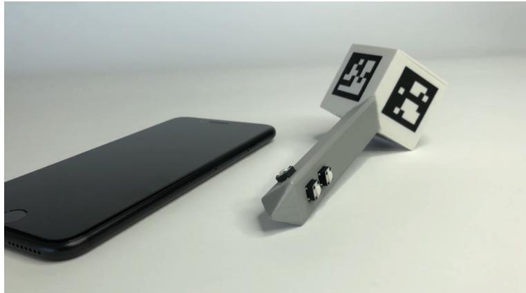
**Figure 3.1:** The ARPen is an input device with three buttons for the input and a box with unique arUco markers at the end.
