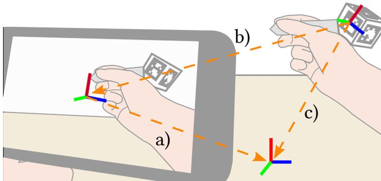
**Figure 3.2:** For calculating the ARPen's position, the position of the smartphone in relation to the AR world's origin is calculated (a). Using the relative position of the ARPen to the smartphone (b), the position of the pen in relation to the AR world can be calculated (c).
