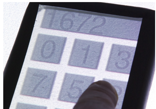
Figure 4: A TaPS Widget covering a PIN entry component. The randomized layout makes it impossible for others to guess the entry from the finger movement.
