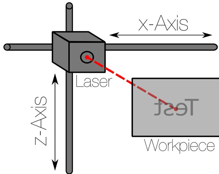
**Figure 3.3:** Sketch of a fixed workpiece (front) and a laser module attached to a 2-axis linear motion system (back).
