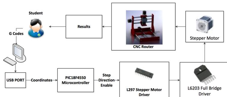
**Figure 2.1:** Educational interaction cycle with a CNC router by Aktan et al. [2016].
