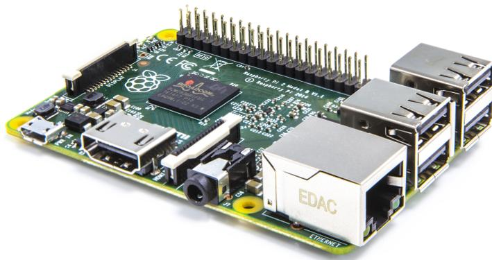
**Figure 2.8:** Raspberry Pi 2 Model B development board
