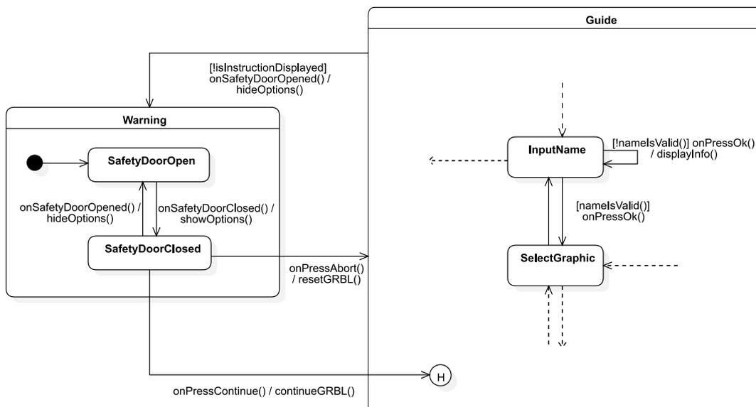
**Figure 3.19:** Incomplete state chart of the relevant GUI changes for the user interaction. Coordination of safety door opening and closing events (left). Name input validation check (right).
