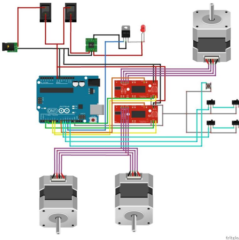
**Figure 2.6:** Schematic of the laser cutter's electronic circuit.
