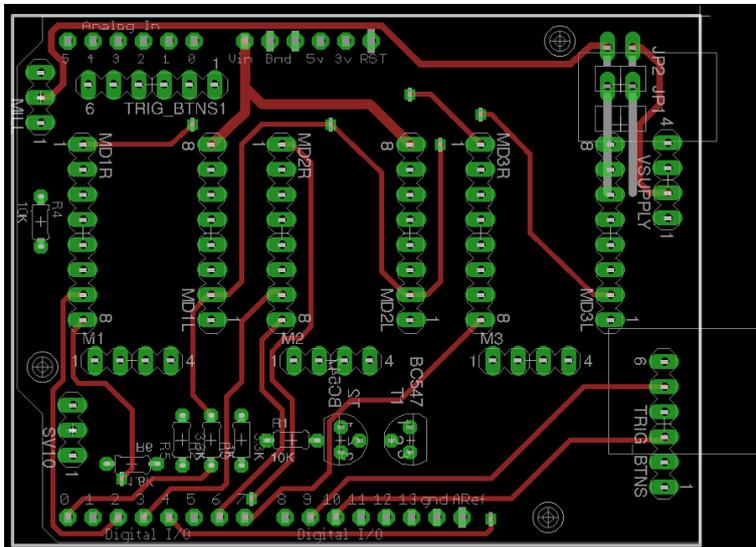
Figure A.2: Arduino Shield Board Layout Top
