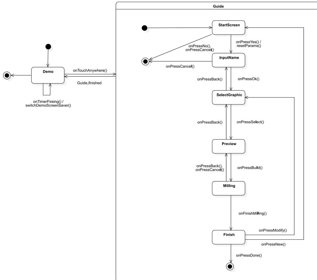
**Figure 3.18:** State chart of the initial GUI functionalities relevant for the user interaction.
