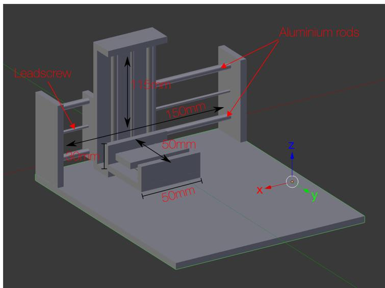
**Figure 3.5:** Rough sketch of the new the linear motion system modeled in Blender.
