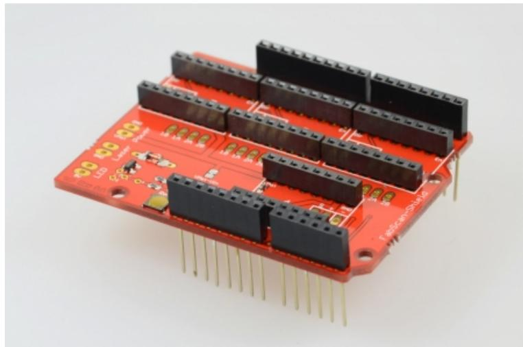
**Figure 2.9:** FabScan-Shield for the Arduino UNO development board.
