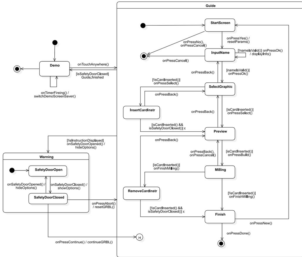
**Figure 3.21:** State chart of the final GUI functionality. The user is now forced to insert and remove the workpiece correctly.
