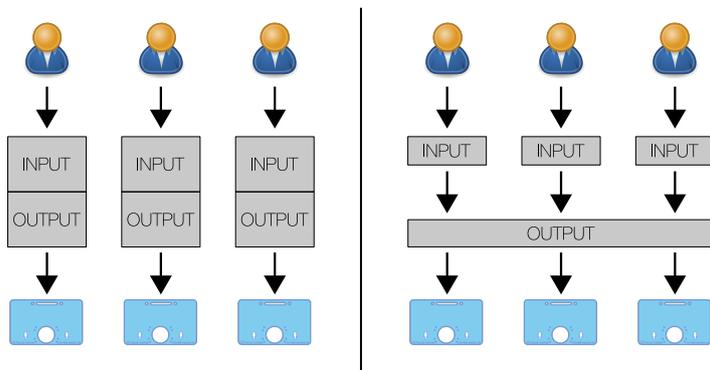
**Figure 5.1:** Two proposals for an increased throughput. (1) Multiple independent devices for each user (left). (2) Multiple clients and one back-end (right).
