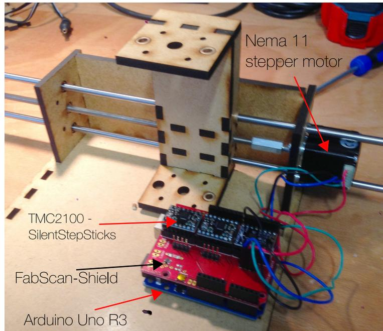
**Figure 3.6:** First implementation of the x-axis system. An Arduino Uno R3 with a FabScan-Shield and three TMC2100 SilentStepSticks are used in order to drive the Nema 11 stepper motor.
