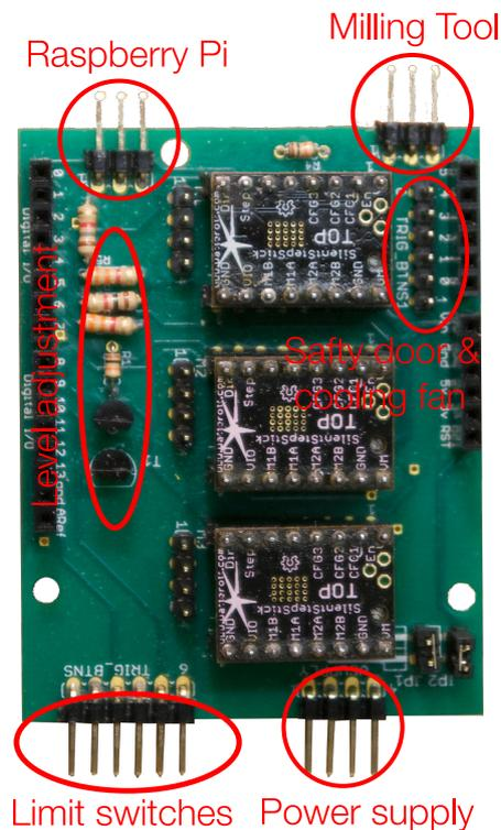
**Figure 3.9:** The new Arduino UNO Shield providing additional pin headers and a power level adjustment.
