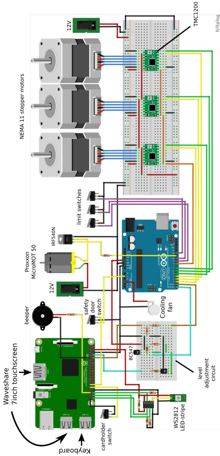
Figure 3.16: Electronic wiring without Arduino Shield
