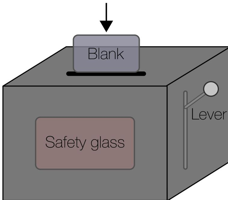
**Figure 3.2:** A card slot affords inserting a card as workpiece into the machine. The lever is used in order to lock the card. The safety glass allows observing the manufacturing process.
