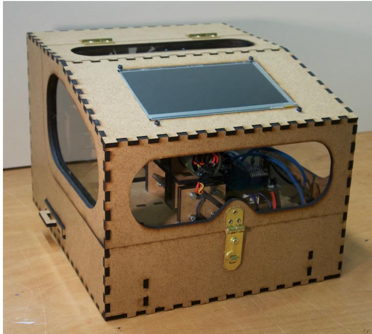
**Figure 3.12:** Exterior view of the assembled device with a case encapsulating the interior milling system.
