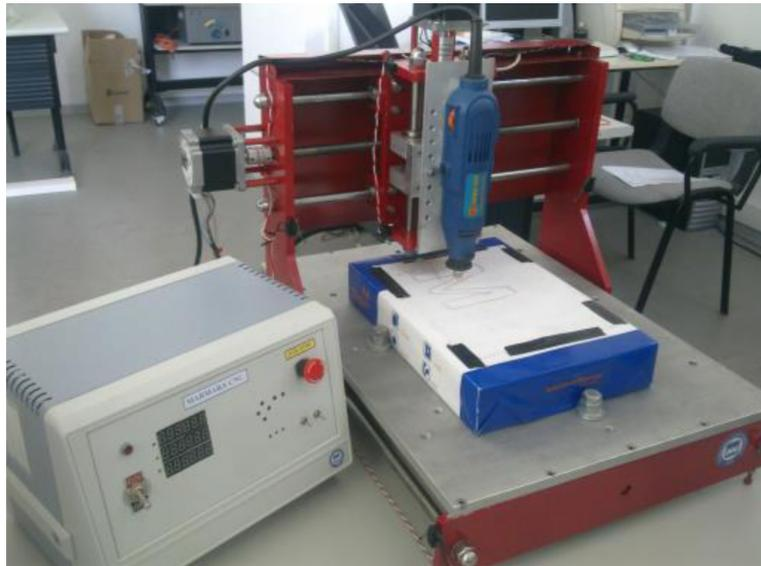
**Figure 2.2:** Control and power supply box (left). CNC router structure (right).
