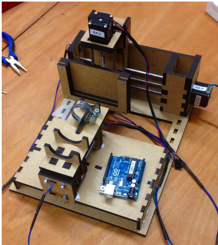
**Figure 3.8:** New linear motion system with the y-axis system placed at the opposite and a movable card holder.
