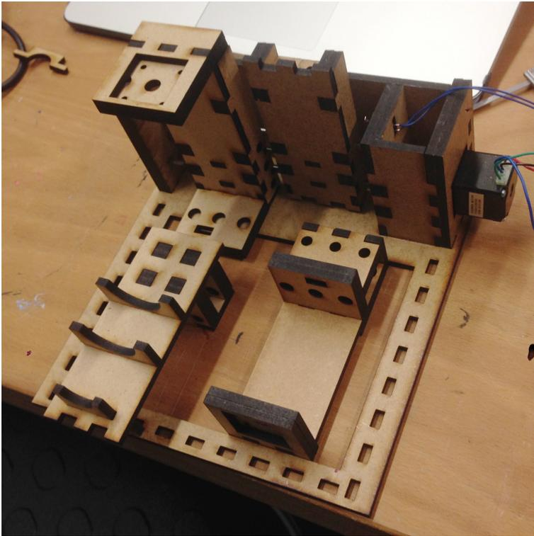
**Figure 3.7:** Components of the adjusted linear motion system with three axes.
