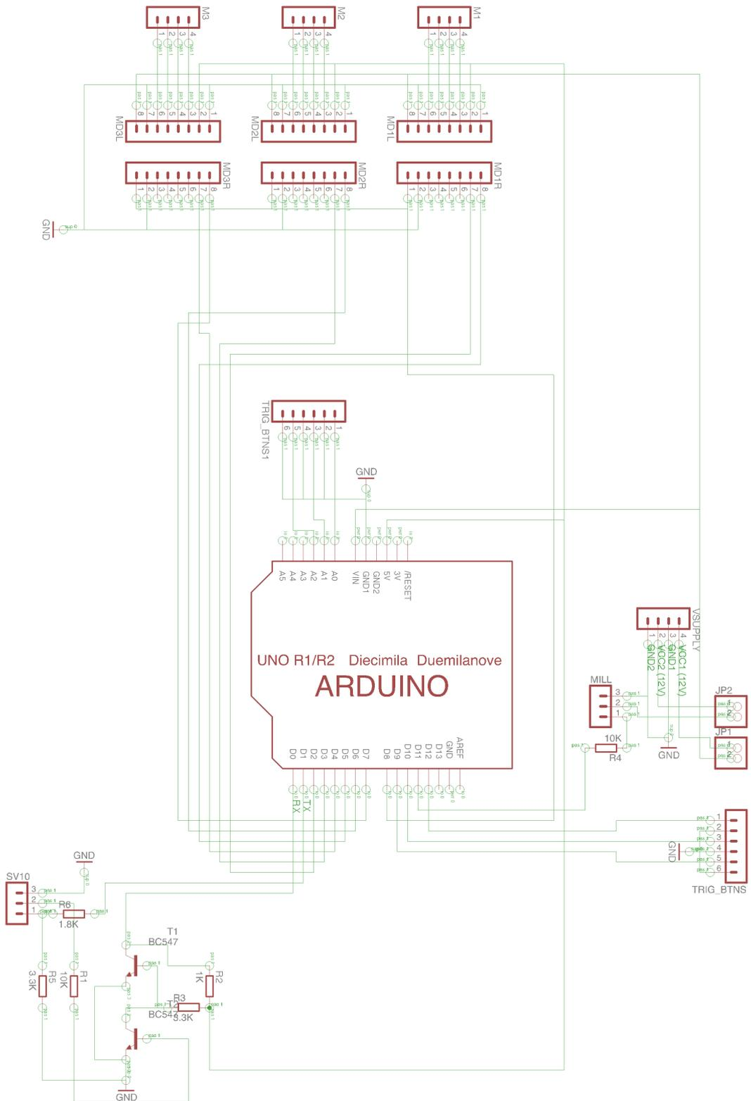
Figure A.1: Arduino Shield Schematic
