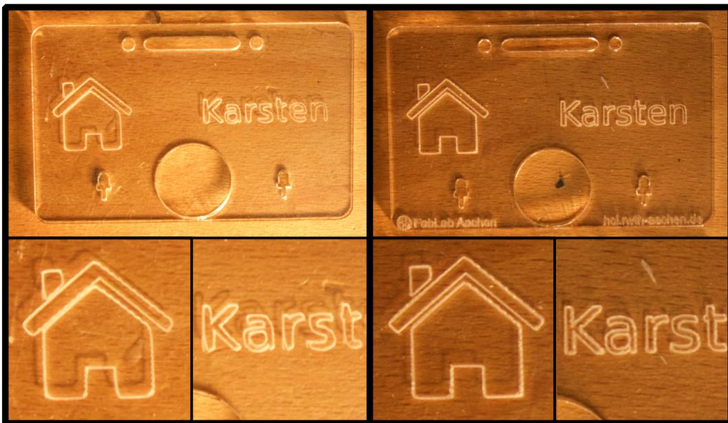
**Figure 3.14:** Name tag engraved by the old prototype (left). Name tag engraved by the new prototype (right).
