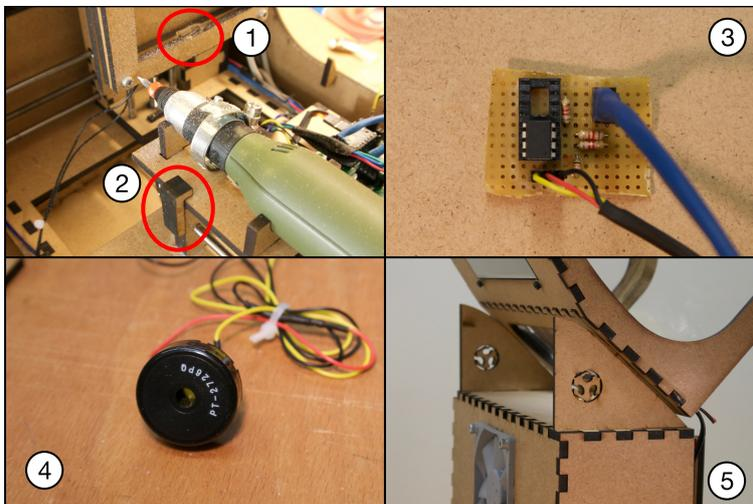
**Figure 3.13:** (1) A microswitch which detects a correctly inserted card. (2) One of the brackets which stabilize the working tool. (3) The ATtiny85 circuit board which drives the WS2812 LED stripes. (4) The beeper connected to the Raspberry Pi. (5) The stand for the safety door.
