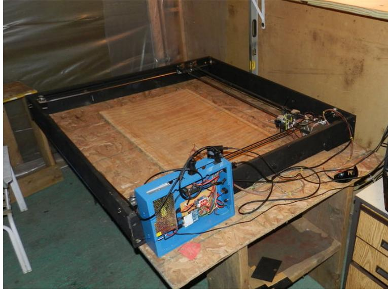
**Figure 2.5:** Blue electronic box in the front of the assembled linear motion system of the 3 watt laser cutter.
