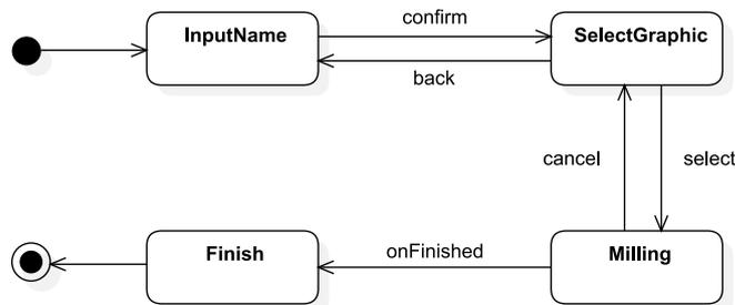
**Figure 3.17:** State chart of the minimal GUI functionality.
