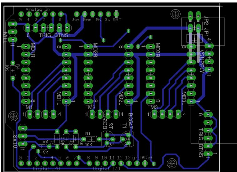
Figure A.3: Arduino Shield Board Layout Bottom
