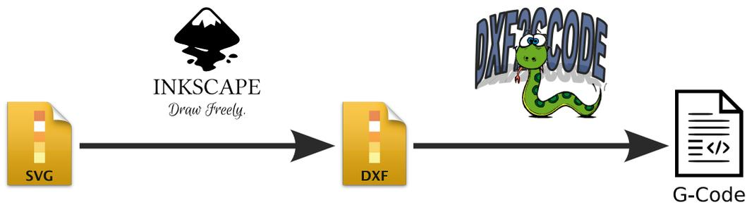
**Figure 3.22:** Conversion from SVG to DXF to G-Code using Inkscape and dxf2gcode python scripts.
