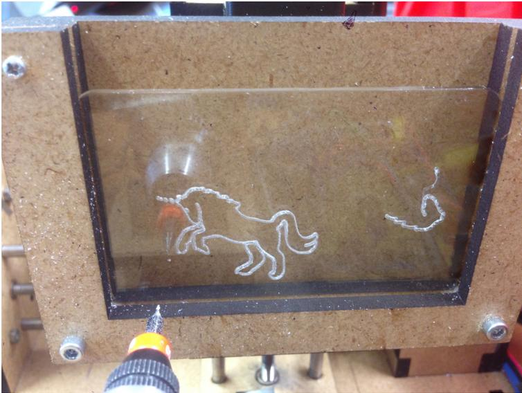
**Figure 3.11:** A unicorn engraved by the milling machine.
