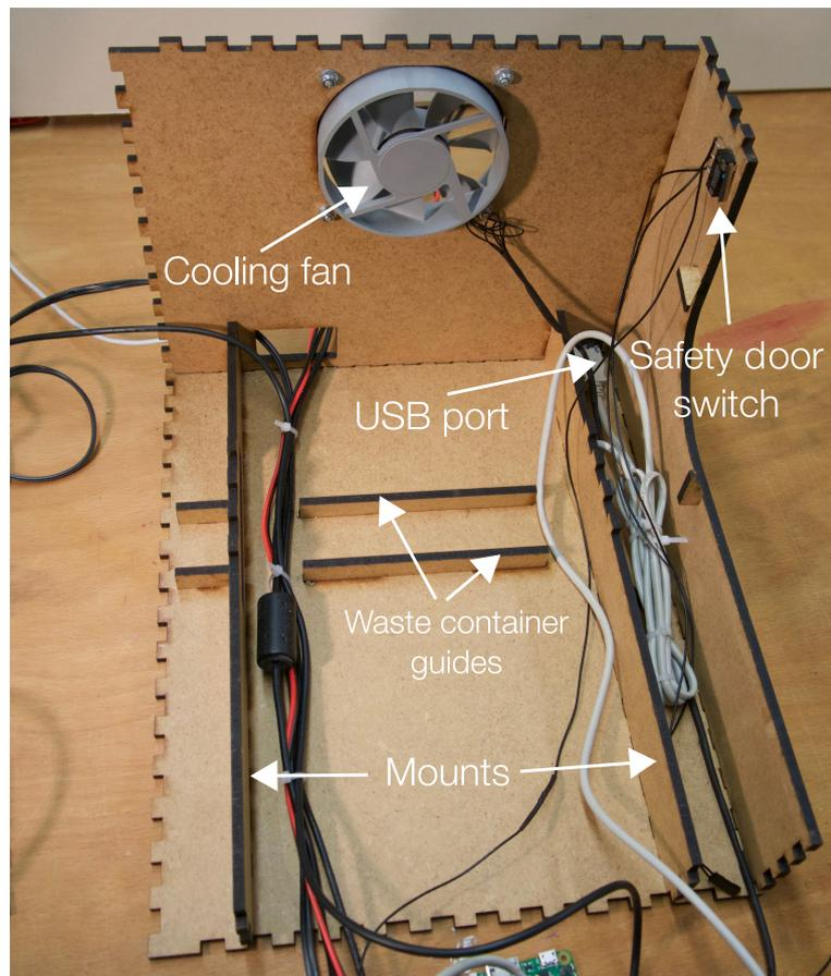
**Figure 3.10:** Interior view of the case and its providing features without the linear motion system.
