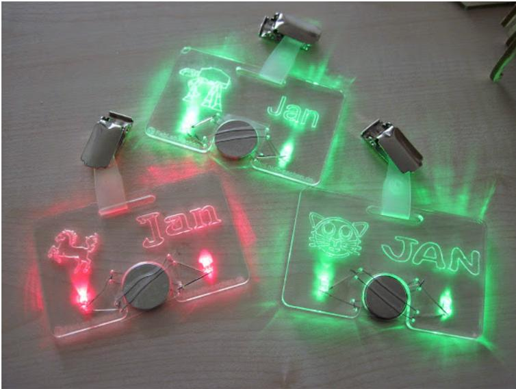
**Figure 1.1:** Three examples of illuminated acrylic name tags which were created using the laser cutter.
