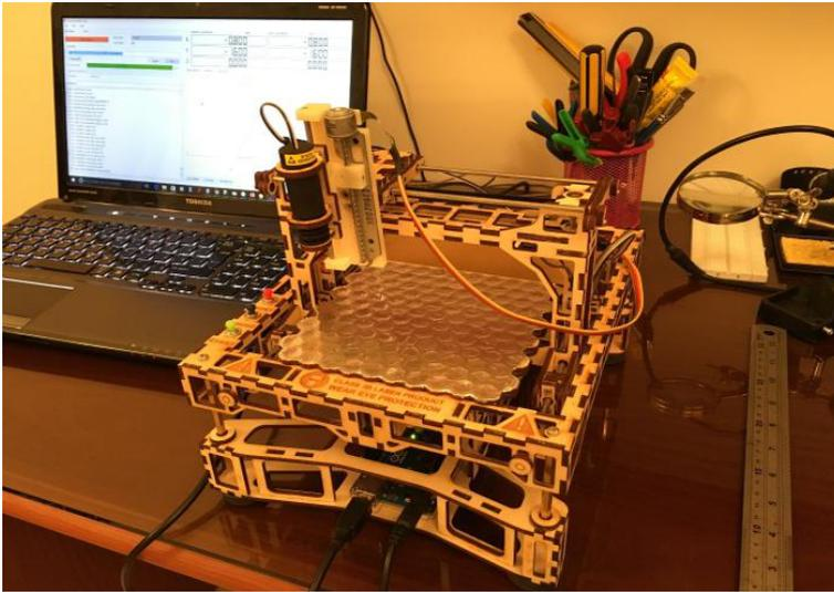
**Figure 2.4:** The assembled portable low-cost mini 3-axis CNC laser cutter.
