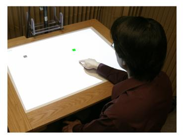
**Figure 2.3:** In Expt. 1, participants used a finger or a mouse to select and drag targets. In Expt. 2, they used either two mice or two fingers to perform a symmetric bimanual docking task (Forlines et al. [2007]).
