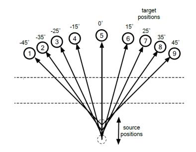
**Figure 4.8:** Experimental design for cross dragging performance task for upward condition (Weiss et al. [2010]).
