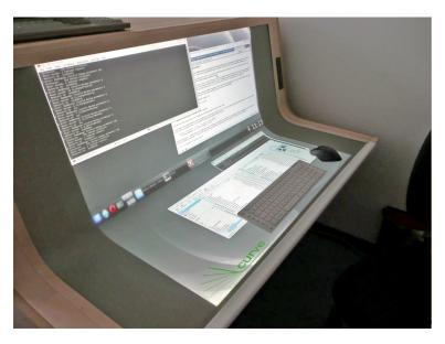
**Figure 2.1:** Curve is a digital desk concept that blends a horizontal and a vertical interactive surface (Wimmer et al. [2010])
