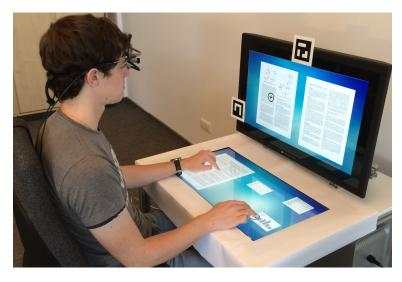
**Figure 1.1:** One can interact on the horizontal surface using direct touch and on the vertical surface using indirect touch with a help of user's gaze.
