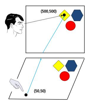
**Figure 3.6:** ITOS mapping example. Blue line indicates the transfer of the touch. The user looks at the object on the vertical screen, touches anywhere on the horizontal screen and her touch is transferred to the object on the vertical screen.
