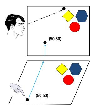
**Figure 3.1:** ITSS mapping example. Blue line indicates the transfer of the touch. User looks somewhere on the vertical screen and touches the point (50,50) on the horizontal screen, which is mapped to the same point on the vertical.
