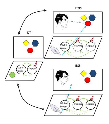
**Figure 3.2:** DT - direct touch. ITSS - indirect touch with an absolute mapping of the input touch. ITOS - indirect touch with a relative mapping of the input touch. Blue line indicates the transfer of the touch.
