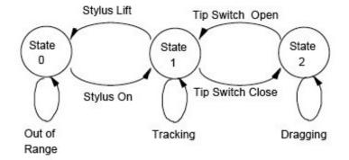
**Figure 2.2:** Three-state model of graphical input (Buxton [1990])
