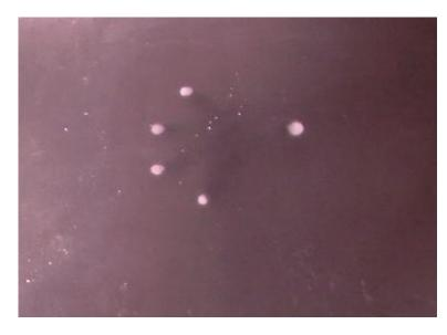
**Figure 2.4:** User touching the multi-touch surface as seen by an infrared-sensitive camera. All five touch points are clearly visible.
