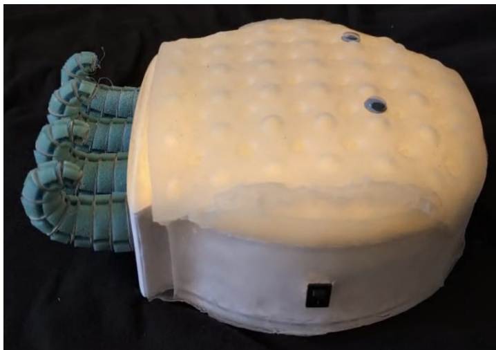
Figure 3.5: Prototype state for happiness/excitement, showing goosebumps, upward-bent tentacles, and yellow light.
