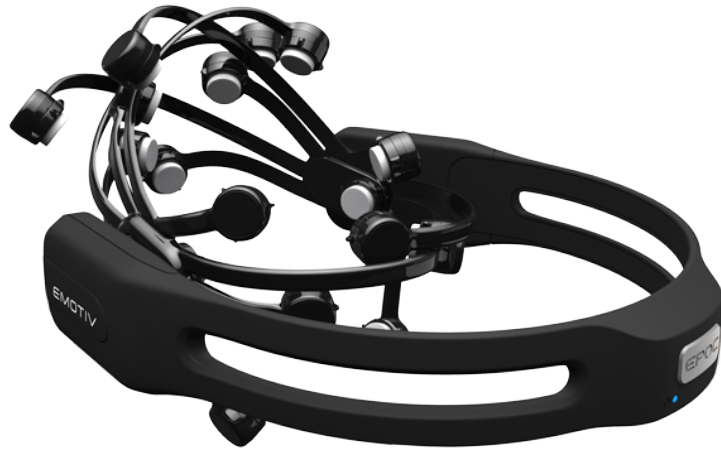
Figure 2.2: Emotiv EPOC EEG headset used for non-invasive EEG signal acquisition in BCI applications [Kaya and Saritas, 2023].
