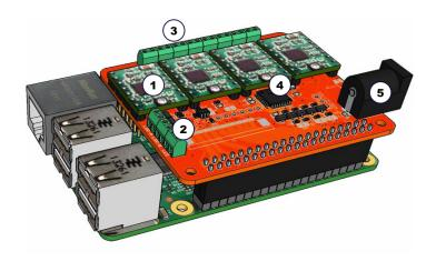
Figure 3.2: FabScan Pi HAT mounted on Raspberry Pi 2
