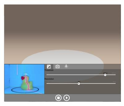
**Figure 3.13:** Settings dialog. Offers the opportunity to find the best scan settings. Left side of dialog: live laser line recognition. Right side of dialog: sliders for changing settings.
