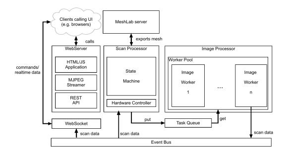
Figure 3.7: FabScan Pi server back-end architecture
