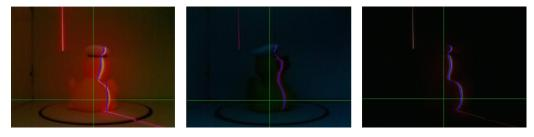
**Figure 3.3:** Different colored filter foils in front of the camera module. Left: without filter. Middle: with blue filter. Right: with red filter.
