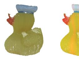
**Figure 3.5:** Scan with different LED light settings. Left: without LED light. Right: with white LED light
