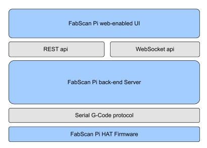
Figure 3.6: FabScan Pi software architecture
