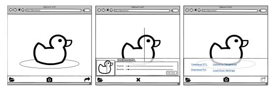
**Figure 3.9:** Mock-up of the web-enabled user interface. Right: Main View, Middle: Settings View, Right: Share View
