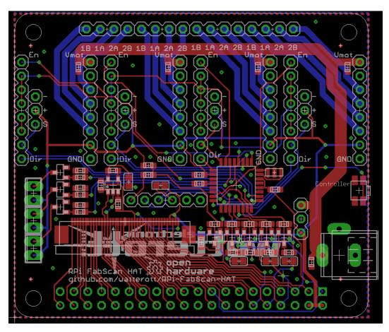
**Figure A.2:** FabScan Pi HAT PCB layout
