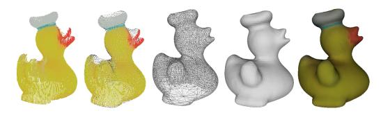
**Figure 3.8:** From left to right. First: point cloud output of FabScan Pi. Second: PLY with mesh reconstruction output of MeshLab, containing colors. Third: meshed STL in mesh view. Fourth: STL with surface, export by MeshLab. Fifth: Exported X3D file with full texture information by MeshLab filter.
