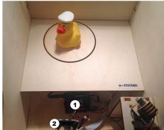
**Figure 3.4:** The final hardware prototype. Left: view from back to front. Right: view from front to back. ① Raspberry Pi with FabScan Pi HAT. ② Raspberry Pi camera module with mounted LED ring.
