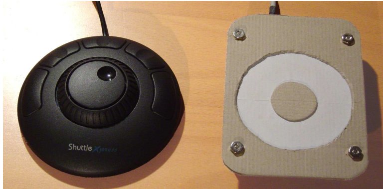
Fig. 4. The ShuttleXpress (left) has an outer self-centering ring for rate control and an inner dial for position control. The Phidgets CircularTouch (right) has a touch-sensitive surface that we used for position control, repackaged to resemble an iPod Click Wheel.
