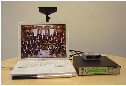
Figure 2. Devices used in our user studies: 14" iBook laptop computer and a Buchla Lightning II baton and tracker.
