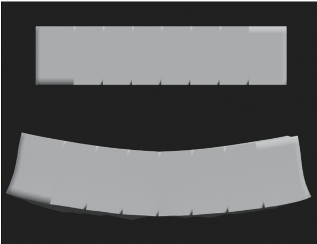
Figure A.3: These images were shown for the first task in the study. Top: An actuator (8 cm x 1.5 cm x 1.5 cm) before actuation. Bottom: The same actuator after pumping air inside.
