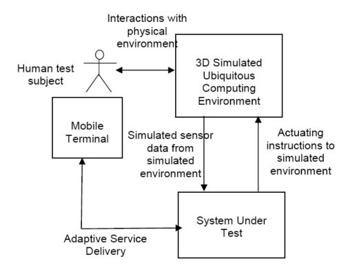
**Figure 2.4:** Tatus system architecture; With extra software the physical device can be used and is not only supported virtually
