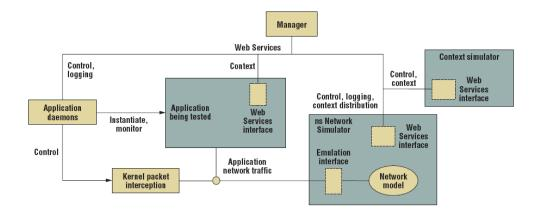
**Figure 2.6:** Setup of the evaluation system; The application code does not need to be changed after the web service interface was implemented
