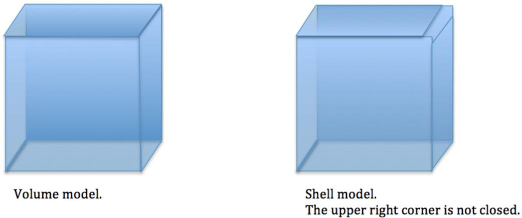
**Figure 2.1:** Example of a volume model (left) and a shell model (right).
