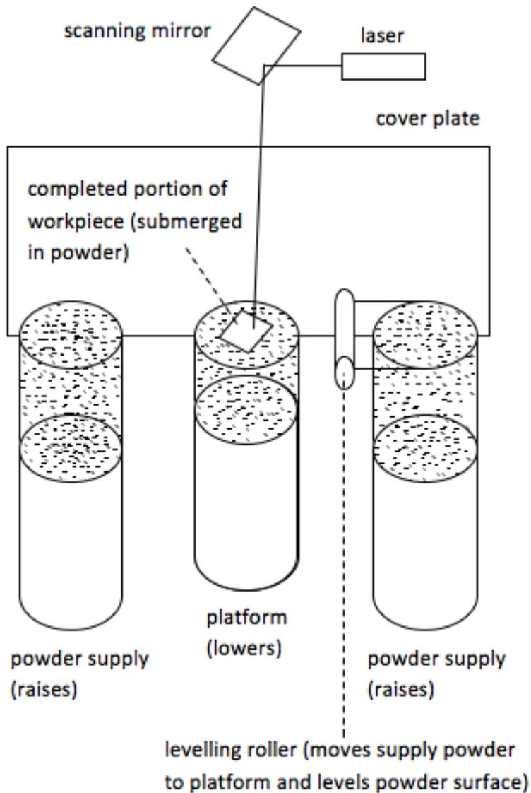
Figure 1.2: Representation of an SLS machine.
