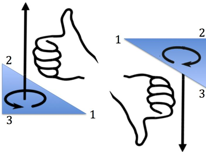
**Figure 2.2:** The right-hand rule defines the orientation of a triangle with the order of its points.
