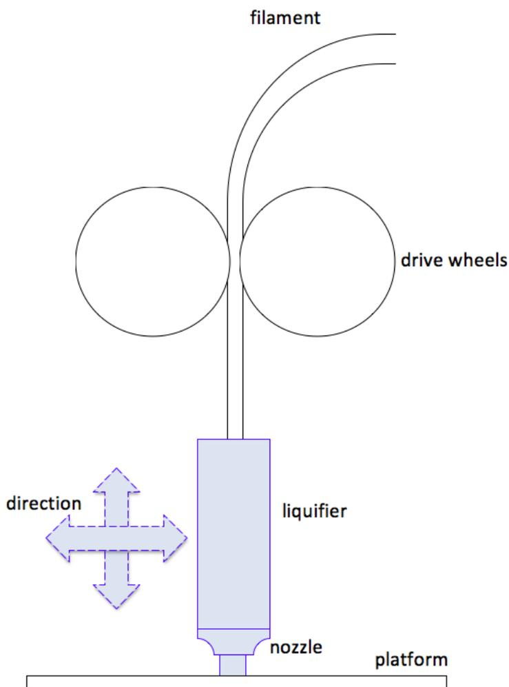
Figure 1.1: Representation of an FDM extrusion head.
