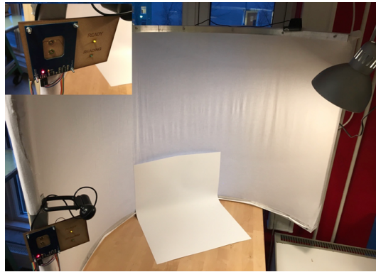
Figure 2.2: The setup of the Protobooth where the prototype must be placed. Lighting and camera setup can be seen along with the system status display on the left [Sjöman et al., 2017].
