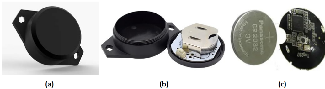
Figure 3.3: (a) The pre-fabricated BLE module we used [Alibaba, a], (b) shows the internal contents inside the black casing [Alibaba, a], (c) shows the arrangement of button cell battery and the circuit board containing all the necessary sensors [Alibaba, b].
