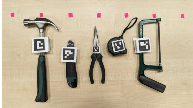
Figure 4.7: Affixing/Tagging tools with different ArUco markers with different IDs to differentiate them.
