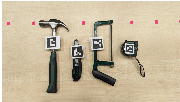
Figure 5.16: The printed ArUco markers with their IDs have been affixed to the corresponding tools respectively.
