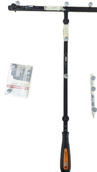
Figure 3.5: The 'wand' along with the custom-made marker arrangements on some tools. It can be seen that the marker arrangements for the pen are not ideal as we are unable to create the distinctive x and y axes needed by the Vicon system to track it in the 3D space. Also, note the need for the objects to be covered in non-reflective tape to avoid unwanted reflections that will cause problems in detection.
