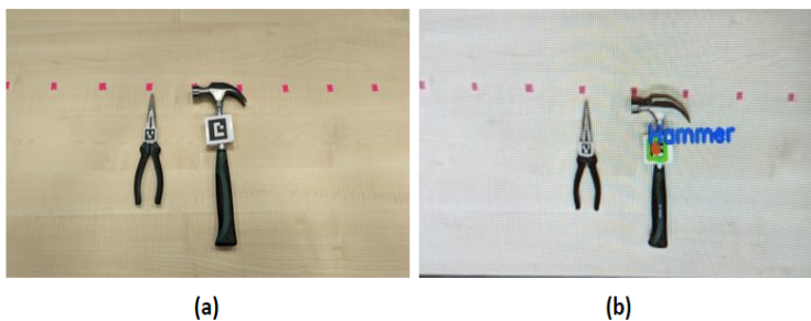
Figure 4.4: (a) The plier uses a marker of size 25mm x 25mm, while the hammer uses a marker size of 45mm x 45mm. (b) The marker of the hammer is detected while the pliers are not, indicating better detections when larger markers are used.
