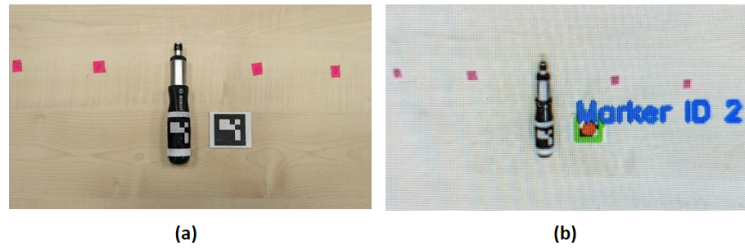
Figure 4.10: (a) Two similar ArUco markers are used. One is affixed on the curved part of the tool ('left') and another is just placed on the table ('right'), (b) 'left' has partial visibility to the camera resulting in a failed detection, while 'right' is detected without any problems.
