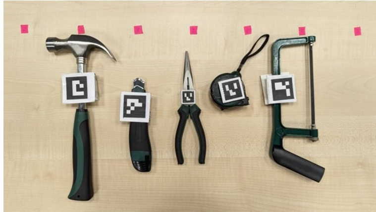
Figure 4.7: Affixing/Tagging tools with different ArUco markers with different IDs to differentiate them.
