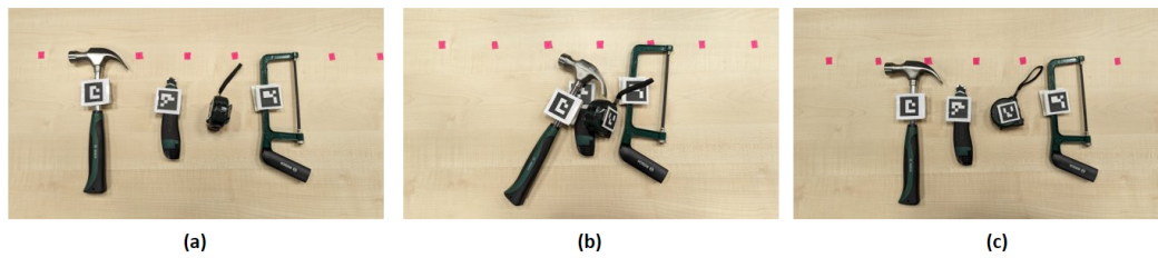
Figure 4.9: (a) The measuring tape is placed on its edge resulting in its marker being obscured from the camera. This must be avoided, (b) Multiple tools are placed over each other again resulting in the obscuring of markers of multiple tools from the camera. This kind of cluttering of tools must be avoided, (c) All the markers are clearly visible to the camera. This is a good practice.
