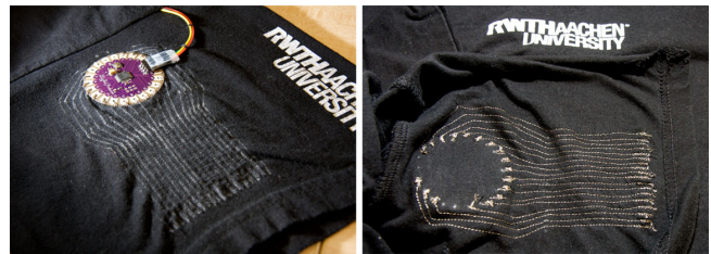
Figure 3: Lines of conductive thread sewn into the sleeve of a T-shirt and connected to a microcontroller board (left: outside, right: inside). Lines are spaced approx. 2mm apart. On the outside, the lines are also painted on for demonstration purposes—normally the black outer cotton thread would be invisible.
