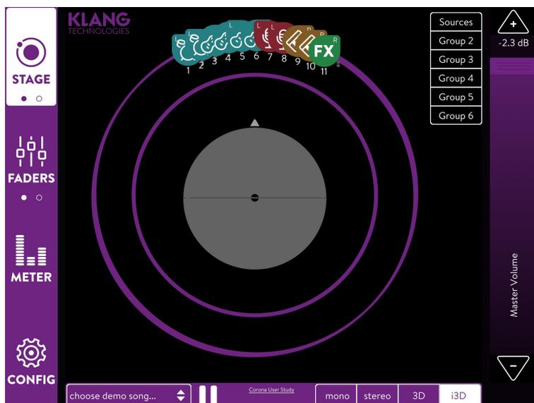
**Figure 3.2:** KLANG:app resp. KLANG:kern Graphical Interface: Here the 11 sources used in the second experiment are shown which are placed with a  $5^\circ$  spacing in azimuth, ranging from  $-25$  to  $25$  degrees.
