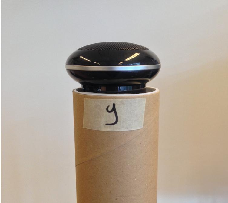
**Figure 3.4:** Sources (cardboard tubes) were numbered and active sources were marked by placing a small loudspeaker on top of the cardboard tube
