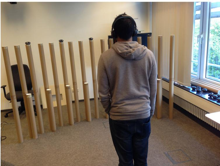
**Figure 4.3:** User standing in front of the arc of cardboard tubes while performing the listening test, in this picture every third tube is marked as active, i.e., an angular separation of  $15^\circ$  was used. The short tubes (70 cm) used for the third condition were half the size of the tall tubes (140 cm).
