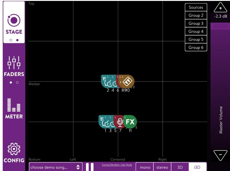
**Figure 4.5:** Sources in the KLANG:kern placed at different heights in the third condition, at  $0^\circ$  (ear-height) and below at  $-45^\circ$ , corresponding to the 140 cm and 70 cm visual source (tube) respectively.
