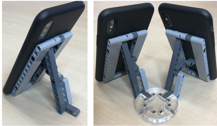
Figure 5.2: The smartphone case (left) has an included stand that can be expanded and collapsed. It ensures that the phone can easily be placed at the correct angle on the table. The connector widget (right) allows the users to arrange up to four smartphones in a fixed arrangement easily.
