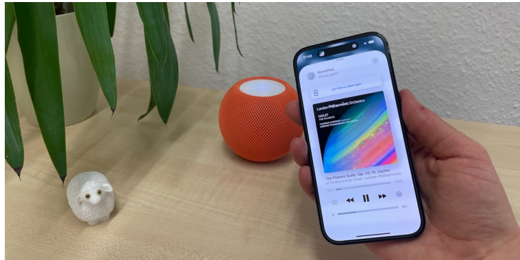
Figure 2.1: An example of spatially aware proximity-based interaction: When an iPhone is held close to a HomePod, it displays an interface to transfer music playback and control the speaker. On the other hand, the iPhone itself is spatially aware of its user and prevents the screen from turning off while somebody is looking at it.
