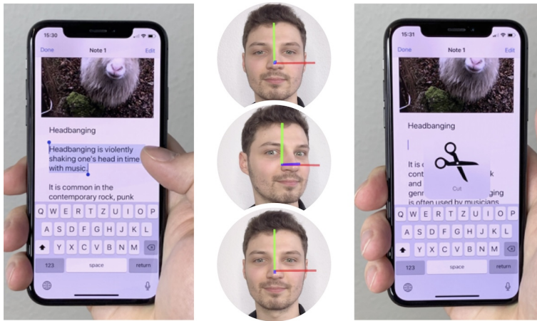
Figure 3.7: In this example, the user selected a part of the text that he wants to cut. After selecting the text with his finger (left), he performs a Handbang gesture to the left (middle) to cut the text (right).
