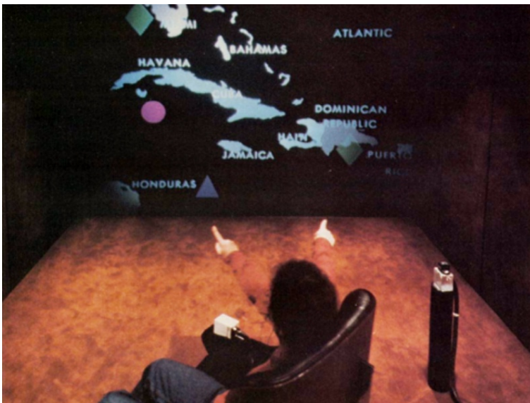
Figure 1.2: Put that There was the first system to support multimodal input. It allowed users to control a cursor by pointing at a location on the screen. Voice commands were used to select elements and activate other functionalities. Image taken from Bolt [1980].
