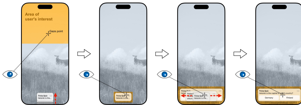
Figure 7.1: Gaze-explicit notifications reduce distraction and occlusion of the primary on-screen content. When a notification is about to be presented (left), the system checks the user’s current gazing location to determine an area of her interest (orange) where no notifications are supposed to appear. The notification then appears on the most distant screen edge. By shifting her gaze toward the notification, a user can enlarge it, revealing more content or additional options.
