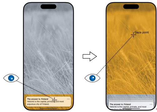
Figure 7.5: Both gaze-explicit as well as gaze-implicit notifications are automatically dismissed when the user moves her gaze away from the notification back to the original position.
