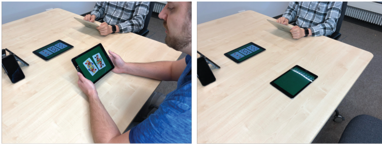
Figure 5.5: GazePoker prevents cheating by continuously authenticating users in front of their cards based on their faces. Those cards are hidden when a player leaves in GazePoker, or somebody else peeks in.
