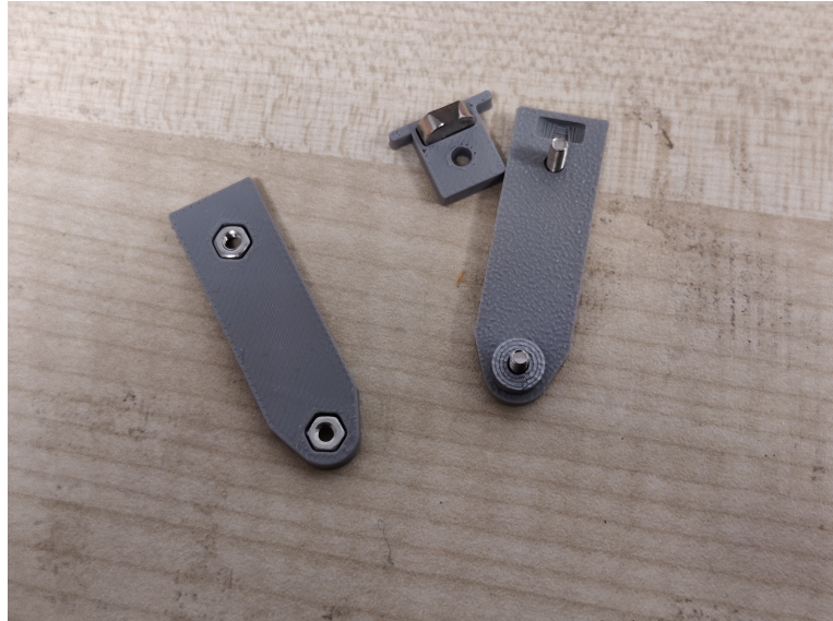
Figure A.8: Image of the piston head components with an inserted magnet.
