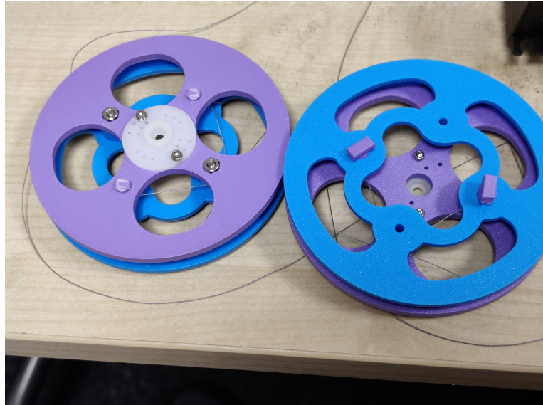
Figure 3.6: 3D Printed spool controlling the strings, with strings mounted to the tensioning mechanism
