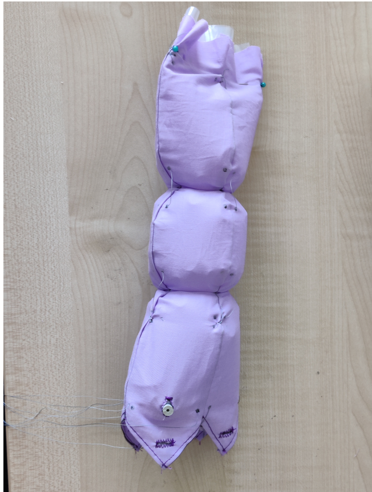
Figure 3.8: Our arm design, using an external fabric layer to cause segmentation
