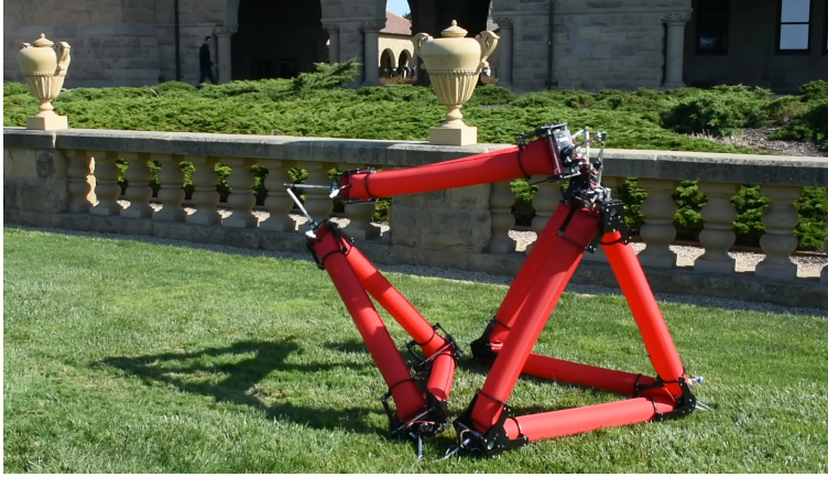
Figure 2.2: Robot based on air-inflated trusses Usevitch et al. [2020]. Image taken from the video 1 .
