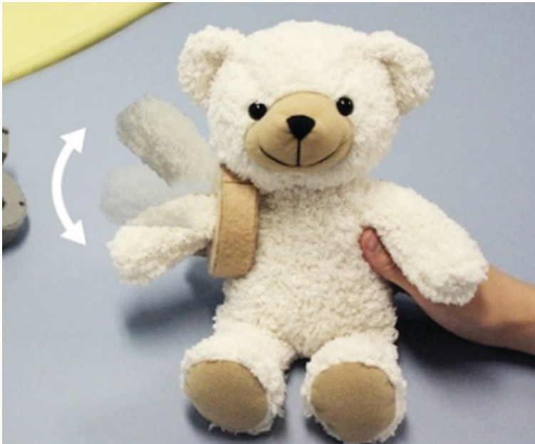
Figure 4.1: Self-actuating teddy bear arm by Sugiura et al. [2016]
