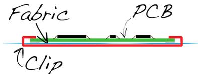
Figure 2: The connection between fabric (blue) and electronics is achieved by a clipping mechanism (red) that presses the ends of the conductive thread against conductive plates on the bottom side of the PCB (green).
