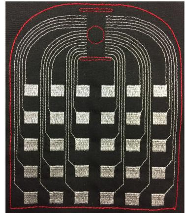
Figure 1: A prototype pattern for an interactive piece of cloth. We measure the interconnections between the patches to get an impression on how the piece is folded. The microcontroller is connected using a clipping mechanism (top).
