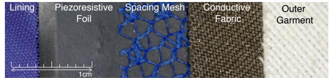
**Figure 2.** FabriTouch layer materials, placed side-by-side to show material structures.
