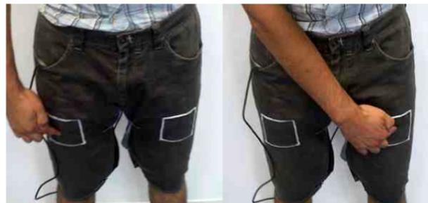
Figure 1. Two FabriTouch pads integrated into a pair of trousers. Users tried both *parallel* (left) and *crossed* touch gestures (right).
