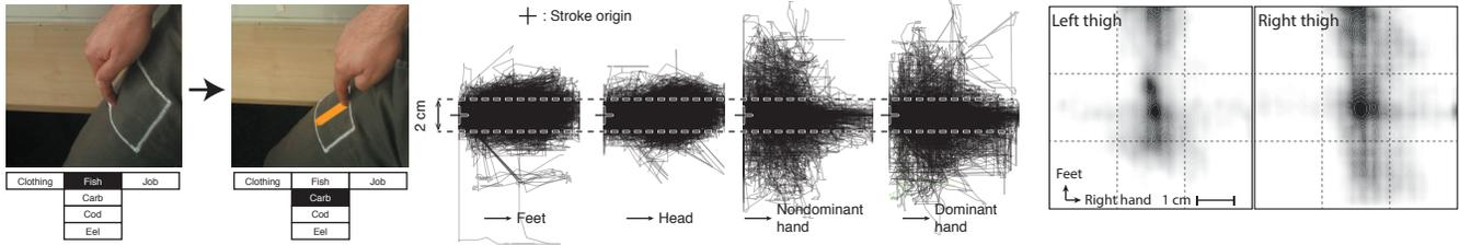
**Figure 4.** Left: Menu navigation mapping in Study 2. A swipe towards the user’s head moves the menu selection downward. Middle: Gesture traces in different directions show high deviation of horizontal swipes towards the nondominant hand. Right: Contour plots show the density of touch locations from Study 2. Users perform gestures mostly in the center third of the touchpad.
