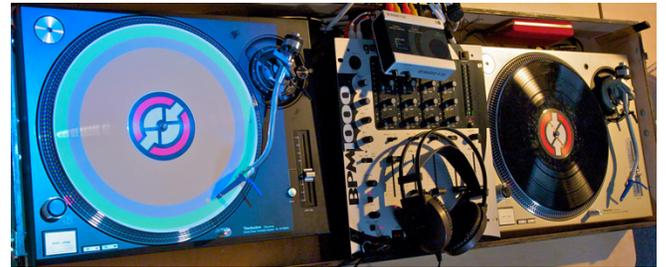
Figure 5. The DiskPlay test setup with the augmented turntable on the left and the traditional timecode vinyl on the right. The projector (not in the picture) is above the left turntable.
