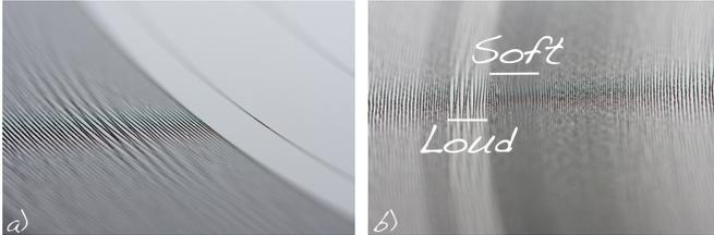
**Figure 2.** Physical structure of a vinyl record. (a) The lead-out at the inner end of the record looks different from the grooves inside the track. (b) Groove spacing varies depending on the volume of the audio signal.
