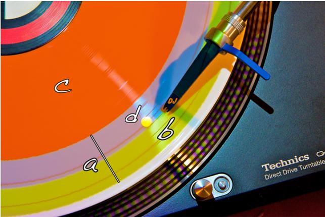
Figure 4. DiskPlay displaying a track. (a) Remaining playback area (blue). (b) Part already played as progress indicator (green). (c) Unused timecode part (red). (d) Cue points (yellow dots).
