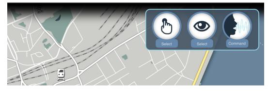
**Figure 3.5:** *Interface 4,* the appearance of this interface is same as *base system.* It only has additional static icons for each modality on top-right corner of the interface.
