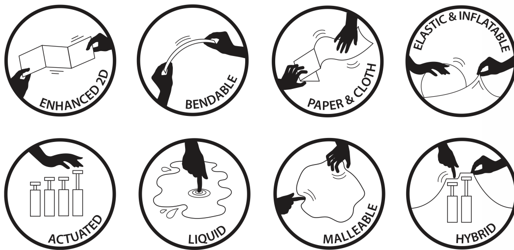
Figure 2.2: The figure shows the 8 suggested categories of shape-changing prototypes. Image taken from Sturdee and Alexander [2018].
