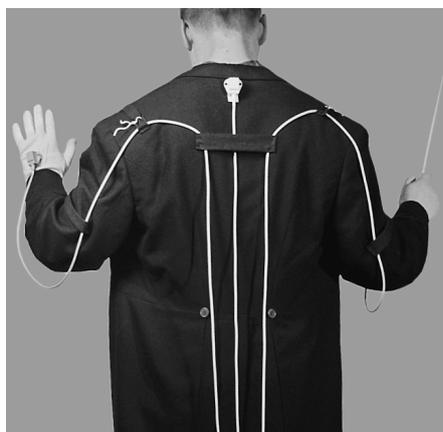
Figure 2.16: DIVA conductor following system sensor placement. Image taken from [Ilm98].
