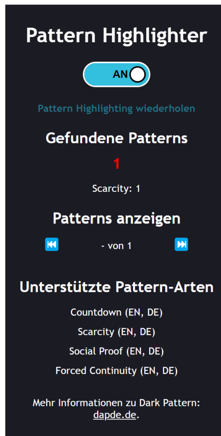
Figure 2.4: Popup of the Dapde Pattern Highlighter a browser extension, including a button to toggle detection on/off and a counter of dark pattern instances found on the respective webpage.
