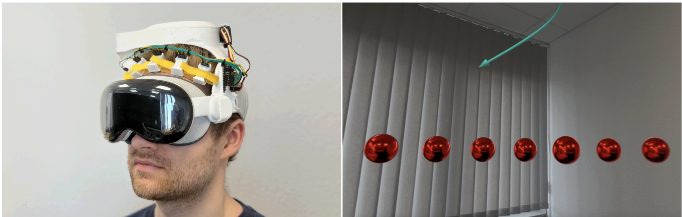
Figure 1: Left: Our head-mounted prototype attached to the Apple Vision Pro. Right: Screenshot of our orientation task with a visual indicator showing which target should be selected.
