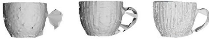
**Figure 3.7:** Surface meshes of the cup. The handle of the cup dramatically increases in quality when using more laser positions. Left: 1 single laser position. Middle: 3 different laser positions. Right: 5 different laser positions.
