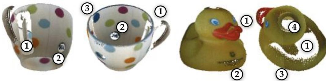
**Figure 3.5:** Point clouds generated with the second prototype from various point of views. Left: the cup. Right: the duck
