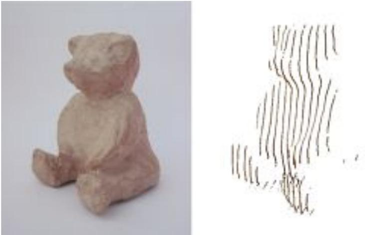
**Figure 3.3:** Scanning results from first prototype. Left: the physical object Bear. Right: the point-cloud of the Bear
