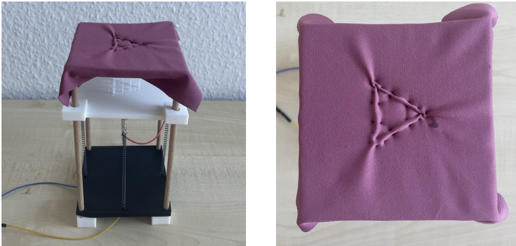
Figure 5.5: This prototype makes use of a stabilization plate to display a single larger triangle.
