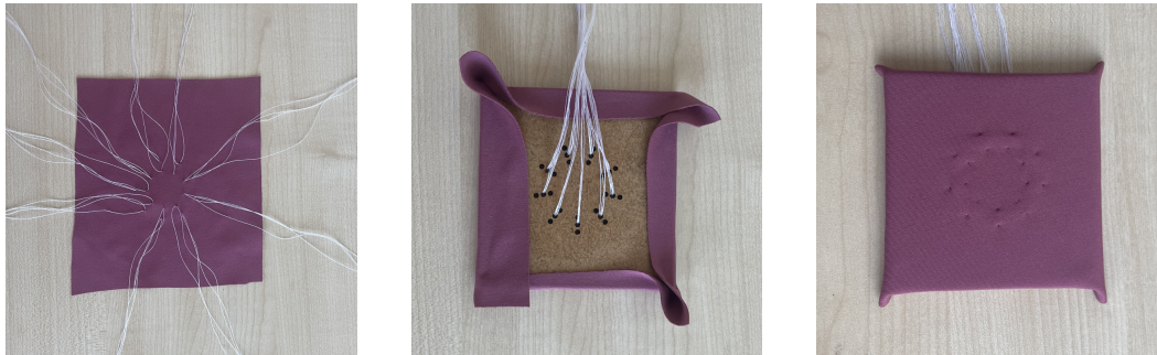
Figure 4.2: Fabricating the Foldlet: Sewing the anchor threads into the fabric, then drawing the strings of one anchor through the respective threading point in the Foam and MDF plate. Finally, glueing the excess fabric in place.
