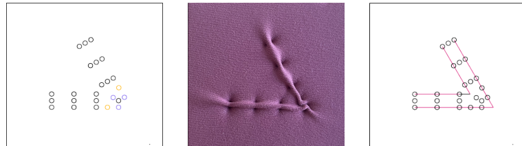
Figure 3.7: The sewing pattern of a 60° Foldlet corner. Left: The pattern of a corner tip, consisting of a 3-anchor (purple) and a 2-anchor (orange). Center: The resulting Foldlet shape. Right: Anchors are aligned to create seamless transitions.
