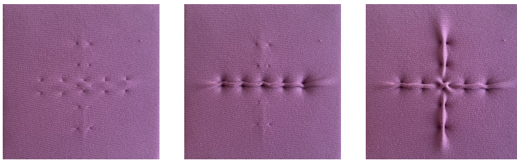
Figure 3.14: An additive Foldlet in stages: No actuation (left), minus icon (center), and plus icon (right). This attempt uses anchors that form a point where the lines intersect.
