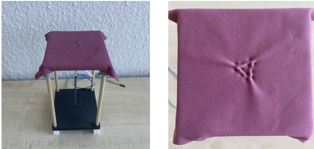
Figure 5.1: Our first prototype uses an actuation stand including a single SMA to activate a small triangle.
