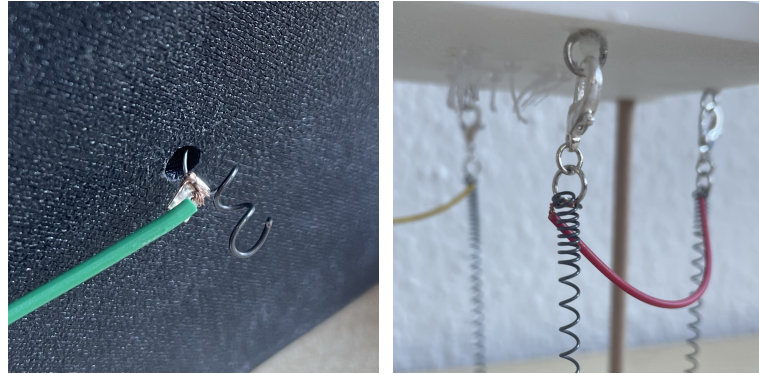
Figure 4.3: Left: Wiring the SMA underneath the actuation stand. Right: Wiring and connecting an SMA to the stabilization plate. We use carabiners to allow easily exchanging between Foldlets.
