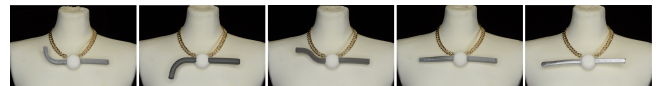
Figure 2: Study 1 investigated how different basic shape change parameters of a necklace affect the emotions it conveys to an observer. When inflated with compressed air, the left actuator changed shape, while the right actuator remained still for reference. Study 1 tested five different motion types (from left to right: bend up , bend down , wave , twist , elongate ). We also varied the appearance of the actuators’ surface material.
