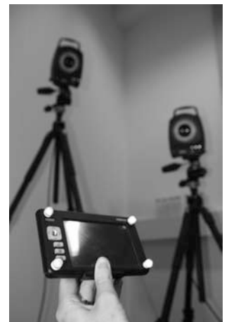
Figure 5 VICON tracking system in the Aachen Media Space to study precise interactions with mobile devices
