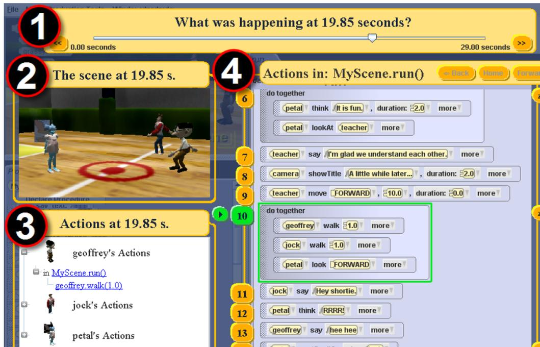
**Figure 3.15:** A sample Looking Glass interface. (1) Time slider for navigating through time. (2) Scene Viewer shows how a scene looks at the selected time. (3) Current Action Pane details what actions characters did at the selected time. (4) Code view selects the executing lines of code. Figure taken from Gross et al. [2010].
