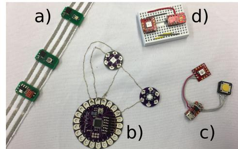
Figure 1. Basic circuit with one button and an LED made with a) YAWN, b) LilyPad, c) Soldered components d) Breadboard.
