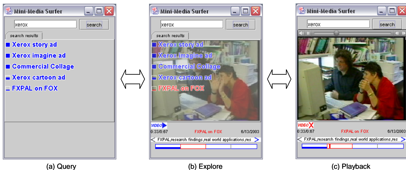
Figure 1. Tasks and transitions: (a) Keyword query and results, (b) Exploration of keyframes from query results, (c) Playback of video segments.
