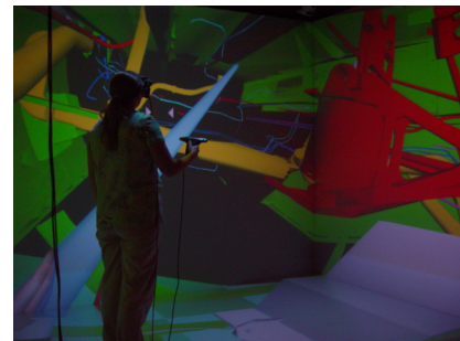
Figure 8: Virtual reality environment displaying airplane components. Complex geometry makes shadow generation costly and shadow interpretation difficult.
