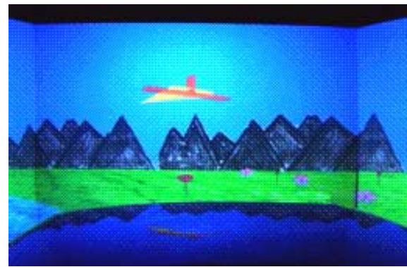
Figure 2. Snapshot of the VGA in the Crayoland virtual environment presented in a driving simulator. The VGA hovered centrally in the middle of the screen and faced the upcoming direction. The lower part of the snapshot is a reflection of the scene on top of the vehicle in the simulator. Subjects sat in the driver’s seat during the experiment.
