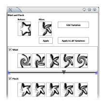
Figure 2. Command dialog boxes are augmented with the capability to add the current result as a new variation (top right button), or to apply the command to all variations simultaneously (bottom bight button).
