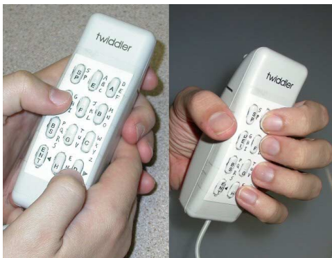
Figure 1: On the left, typing using multi-tap on the Twiddler keypad. On the right, chording with the Twiddler one-handed keyboard typing the letter ‘s’ (M0L0).
