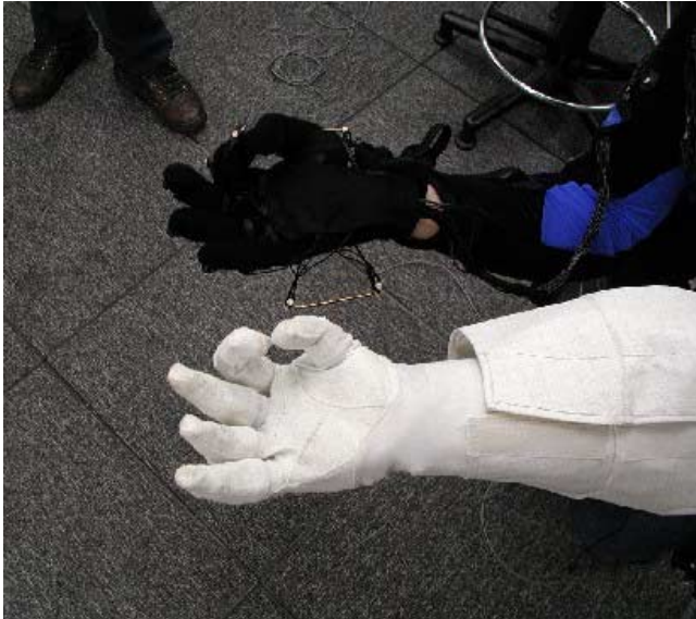
Figure 7: Cartesian control using prototype optical glove
