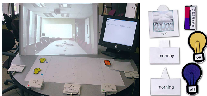
Figure 4. SiteView, a spatial UI for end-user control of home automation systems. Left: A physical light-bulb icon on the floor-plan, with projected feedback above. Right: The six physical icons.
